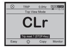
2 If you press the [STOP/RESET] key again while "CLr" is blinking, the trip is reset.
